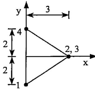
5. The face containing nodes 1-4-2-5-3-6 of a 10-node tetrahedron element coincides with  $z = 0$  plane as shown. This face is subjected to uniform traction  $p_z = p$  in  $z$  direction. Use volume coordinate or area coordinate to calculate the consistent loads in  $z$  direction for all 10 nodes. (20%)
