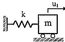
Figure. 2 (Given mass  $m = 10 \text{ ton}$ , spring constant  $k = 640\pi^2 \text{ kN/m}$ )
