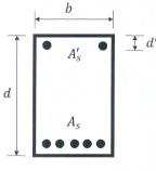
$\frac{1}{4} d' \quad \rho = A_s/bd$   $\rho' = A'_s/bd$  d'/d = 0.1  $f_y = 40 \text{ ksi } (276 \text{ MPa})$   $E_s = 29 \times 10^3 \text{ ksi } (200000 \text{ MPa})$
