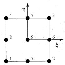
5. A linearly varying distributed load acts normal to an edge of a four-node plane element. Calculate the consistent (or equivalent) nodal loads at nodes 1 and 2 in y direction. (15%)
