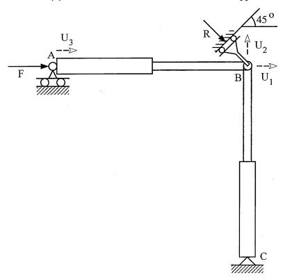
(d) In (c), if the horizontal displacement of node A is  $U_3 = 0.1$  in, calculate the displacements  $U_1$  and  $U_2$  of node B, the magnitude of force F applied at A, and the reaction R at the skew roller support. (10%)
