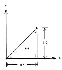
(3) Show that the bilinear interpolation functions for the four-node triangular element in Fig. 3 are of the form (20%)
